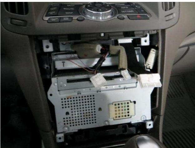
23. Install the 2 screws at the bottom of the screen bezel which holds it in place. Connect the radio/climate control connectors and reinstall the controls. Install the 2 screws and reinstall the cover that goes under the controls.
