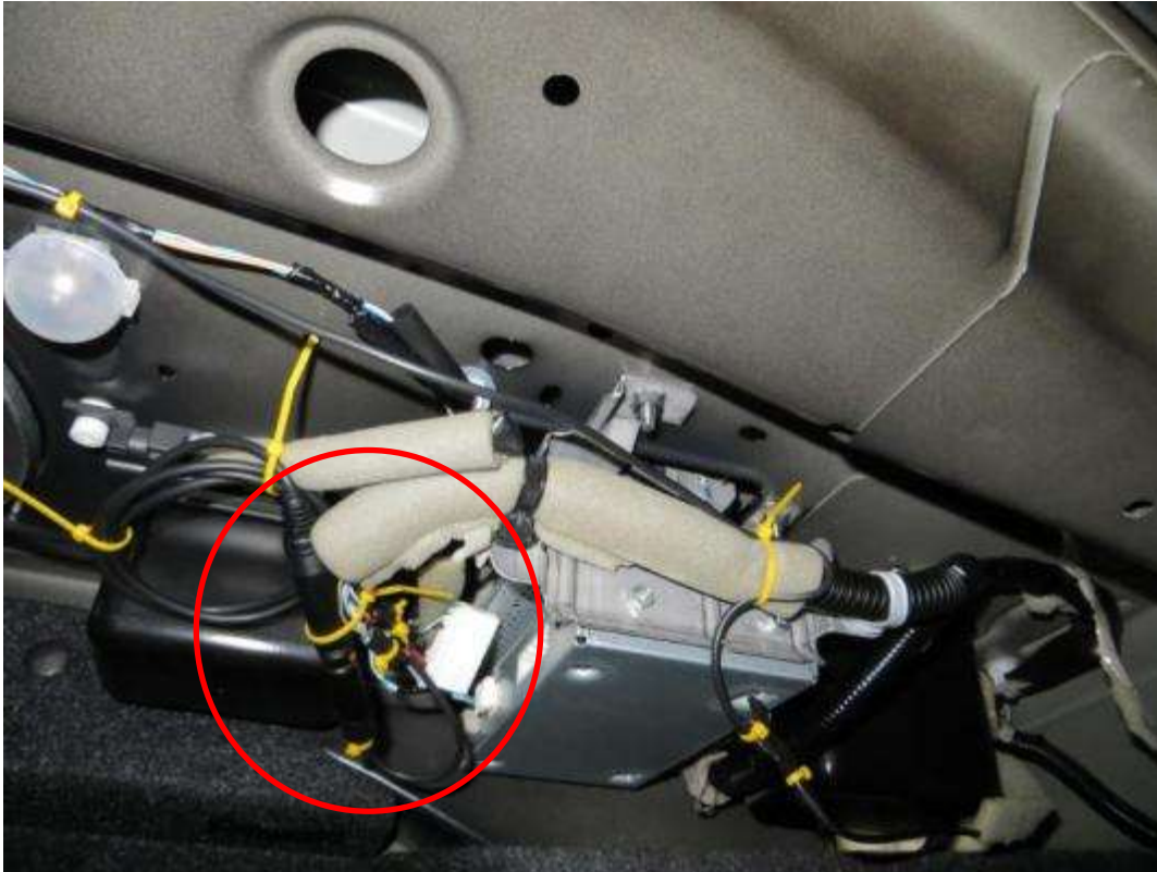
M210 connector with male connector (MAKE SURE GROUND GOES TO GROUND, SIGNAL GOES TO SIGNAL, ETC):
